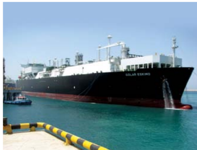
The Floating Storage and Regasification Unit (FSRU), 'Golar Eskimo'.
